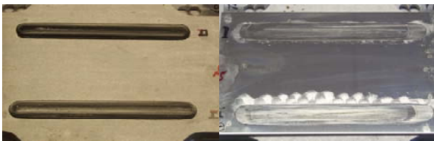
pict. 8: MSM®-strips after a sliding path of 10,000 m
