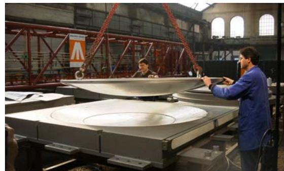
Fig.21 : SI - sliding isolator for 130,000 kN load (SLS)
