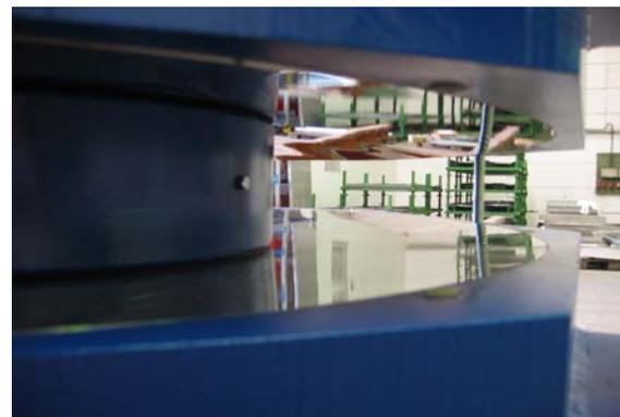
Fig.23 : Double sliding isolation pendulum (SIP-D)
