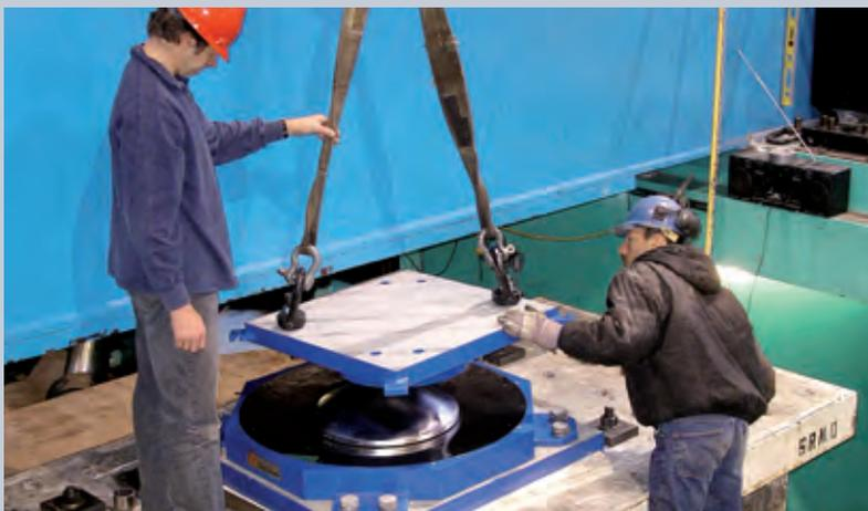
SIP bearing installation at the shake table of the seismic test laboratory of the University of California in San Diego, USA. Here to be seen the special calotte with its 2 curvatures above and below.
