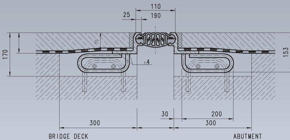
Low cost elastoblock joint can be used in cases where no vulcanisation of mats is required.
